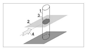
Figure 1. View of the object under aerodynamic analysis: 1 – long cylinder, 2 – DVM analysis plane, 3 – section from Fig. 3, 4 – wind attack
