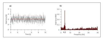
Figure 3. Side forces affected by the cylinder from Fig. 2: a) time history of the force b) amplitude spectrum
